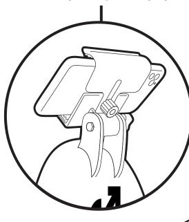
Install top cell phone cradle with supplied bolt and wingnut
